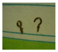
Left: after bending; Right: before bending
